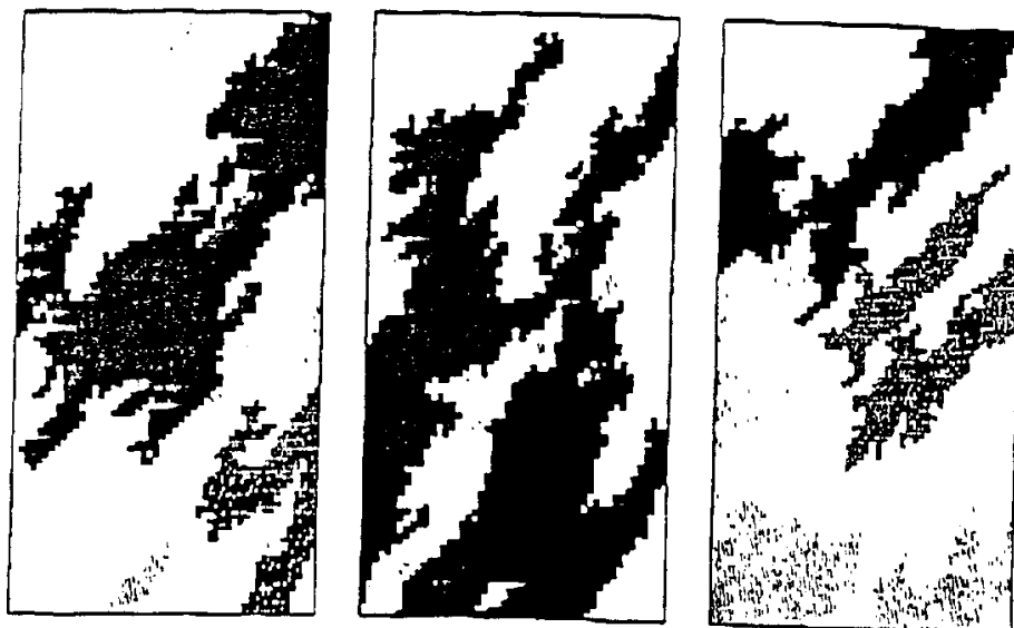
Figure 10.10: Slices through three facies models. The black region on each realization is the largest geo-object. Smaller geo-objects are shaded in gray.
